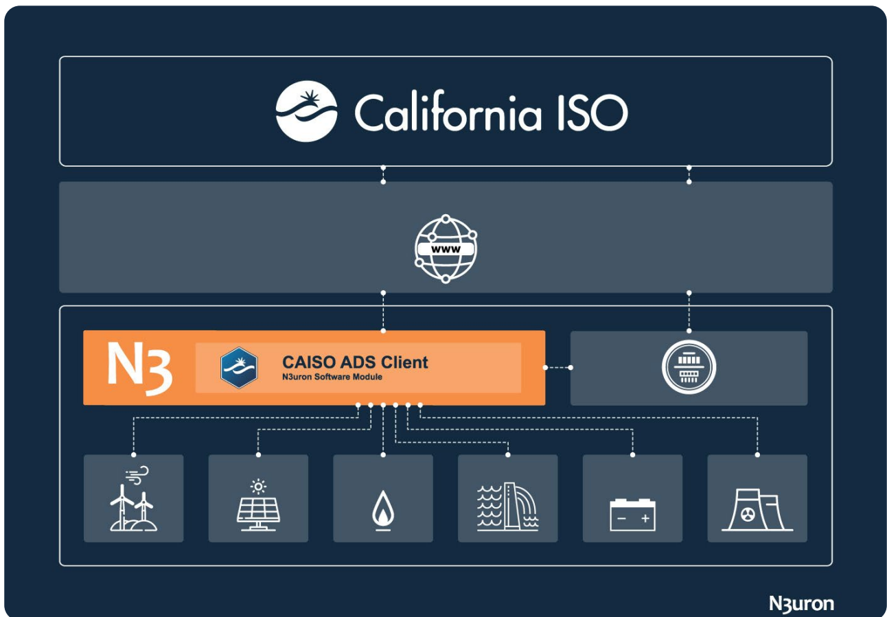
Diagram displaying how the CAISO ADS Client module allows receiving, scheduling and executing CAISO ADS requests.
